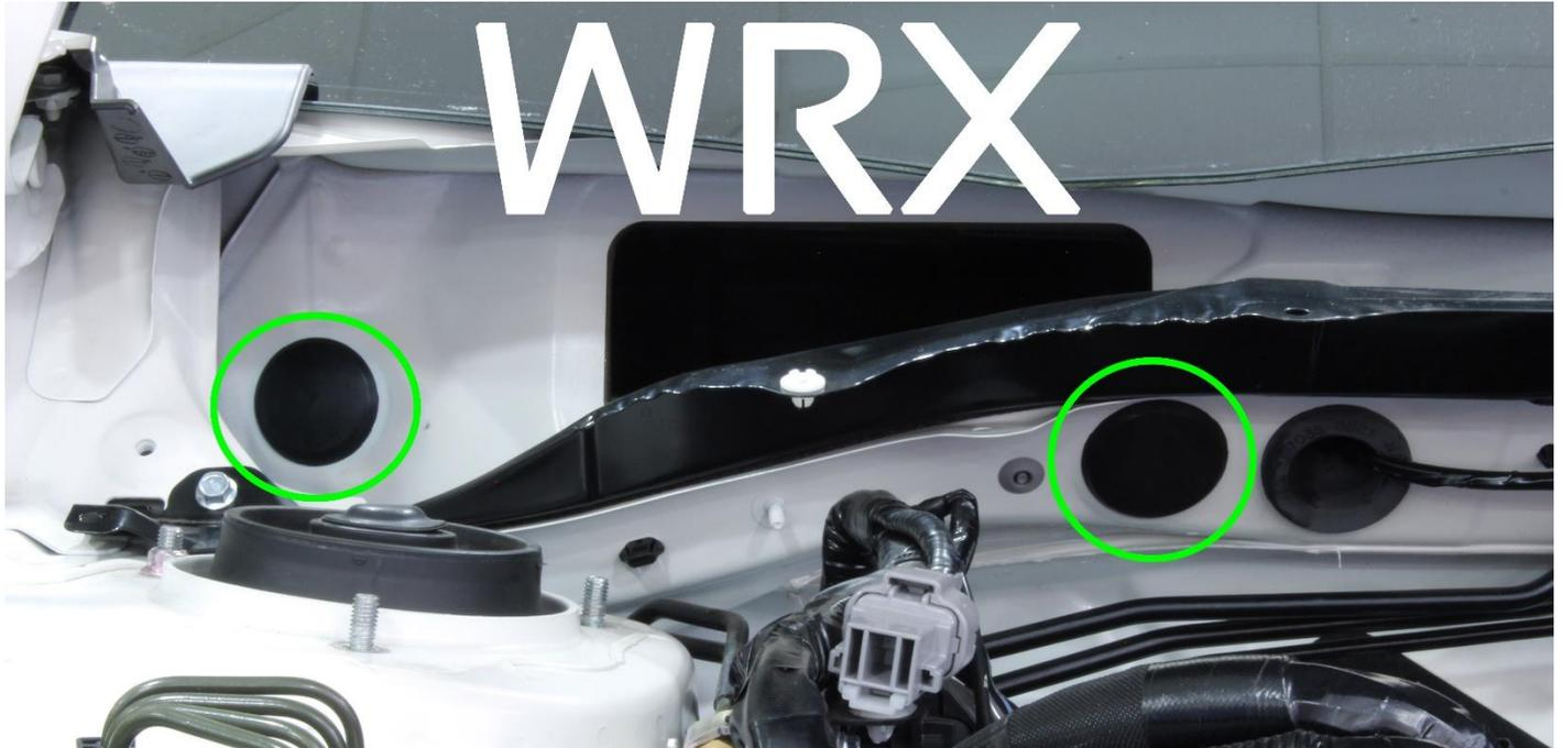
Above picture shows both engine bay firewall plug (right side of picture) and second plug located behind plastic windshield wiper cover (left side of picture).
