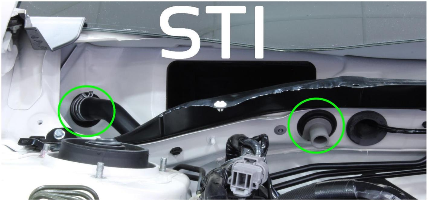
Above picture shows both engine bay firewall grommet (right side of picture) and grommet located behind plastic windshield wiper cover (left side of picture).
