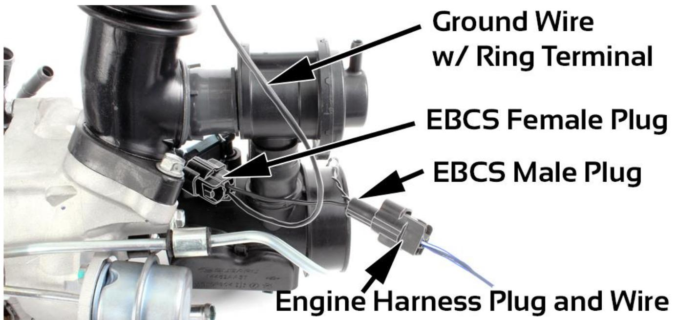
18. Locate engine ground on right side engine head. Remove 10mm bolt (with OEM engine ground still on bolt) and place ring terminal from EBCS Pro harness on bolt, then reinstall back to head. **NOTE: Both the OEM and EBCS Pro harnesses will be grounded using same bolt.**
