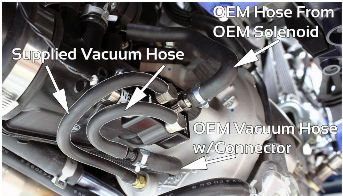
13. Remove "Tee" from vacuum hose going to wastegate actuator and discard remaining hose. **NOTE: This hose is shown in picture above indicated with "OEM vacuum hose w/connector".**
