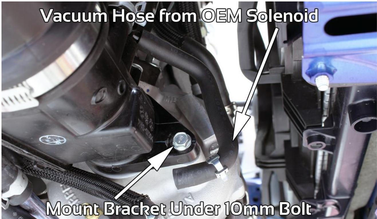
8. Using supplied M8 washer and M8 button head bolt, secure EBCS to bracket as shown in pictures, making sure to face side with (3) ports toward front of car. **NOTE: Orientation of EBCS and bracket may need to be adjusted in future steps.**
