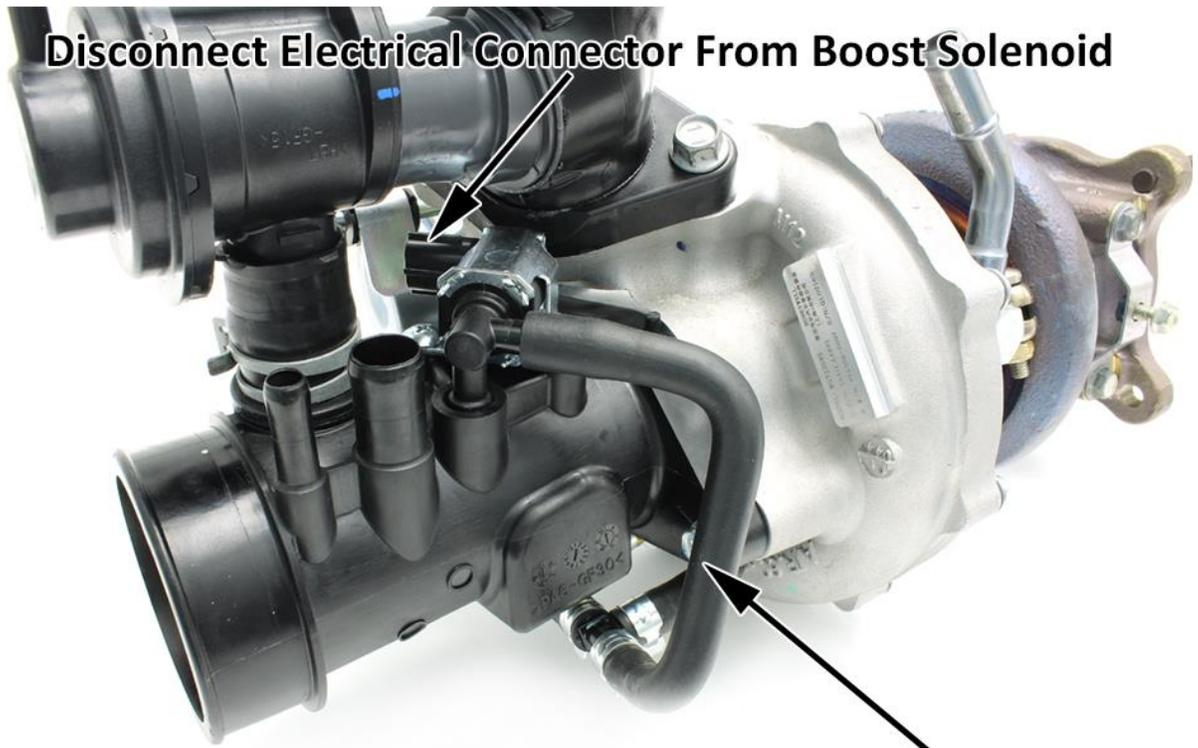
6. Locate vacuum hose coming off solenoid (see arrow in picture above), and remove from "tee" junction on lower side of turbo.
