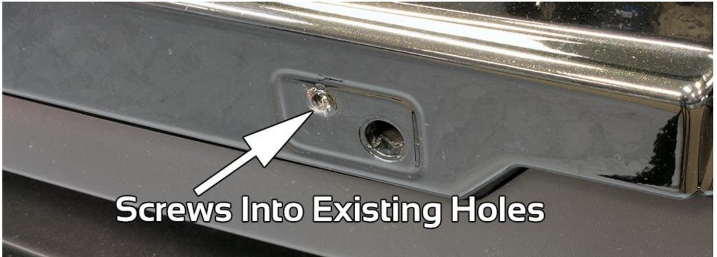
3. Decide which side of plate you want showing and using supplied screws, mount plate to car.
