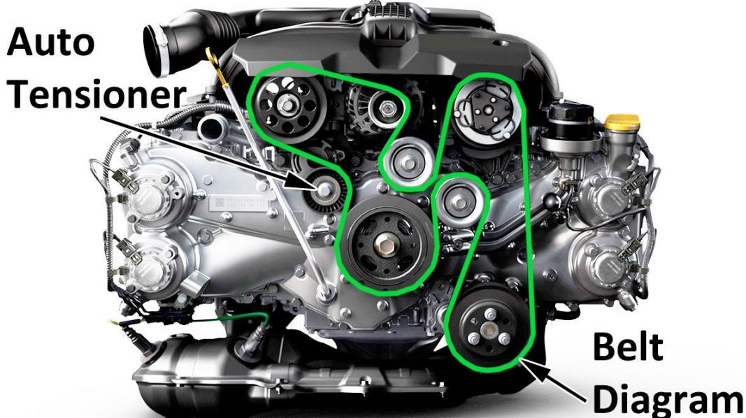
Above Diagram for FB Engine (2012+ Impreza), FA engine (BRZ/FR-S) has similar routing except upper middle pulley is missing.
