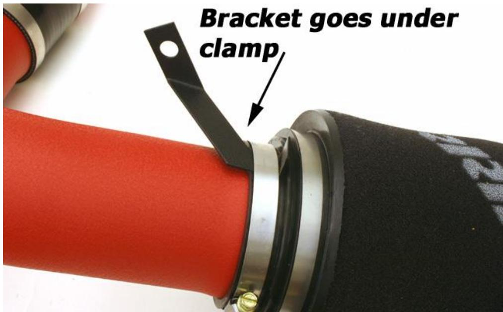
18. Adjust all pieces of the intake system to align pieces for best fit. When aligned, tighten all clamps. **NOTE: some alignment of tubes may be needed after a test drive to ensure no parts are coming in contact with chassis.**
